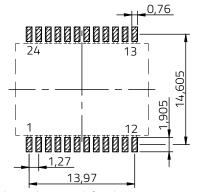
Unless otherwise defined tolerance: ±0,10mm no vias or traces underneath the component
