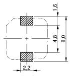
no sensitive traces underneath the component
