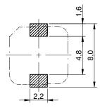
no sensitive traces underneath the component
