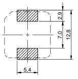
no sensitive traces underneath the component
