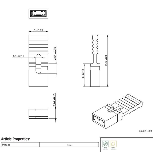
CHECKED REVISION DATE (YYYY-MM-DD) GENERAL TOLERANCE PROJECTION METHOD Ð CPo 004.000 2023-07-24 DIN ISO 2768-1m DESCRIPTION **WR-PHD Jumper with Pullback** ORDER CODE 609002115121 SIZE/TYPE STATUS BUSINESS UNIT PAGE 1/5 2.54 mm eiCan Valid
