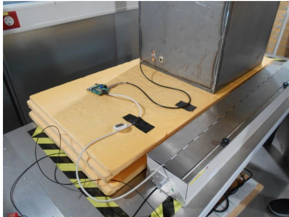
Figure 22: Setup for burst testing to determine the maximum test level
