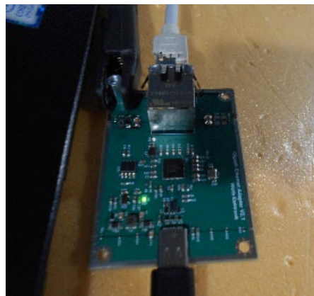
Figure 35: Test setup for direct surge coupling into the cable shield with 2 Ω generator impedance. Surge decoupling by means of an alligator clip and metal bolt on the level of the Ethernet jack – in the picture above left
