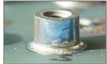
Soldering result: incorrect coating
