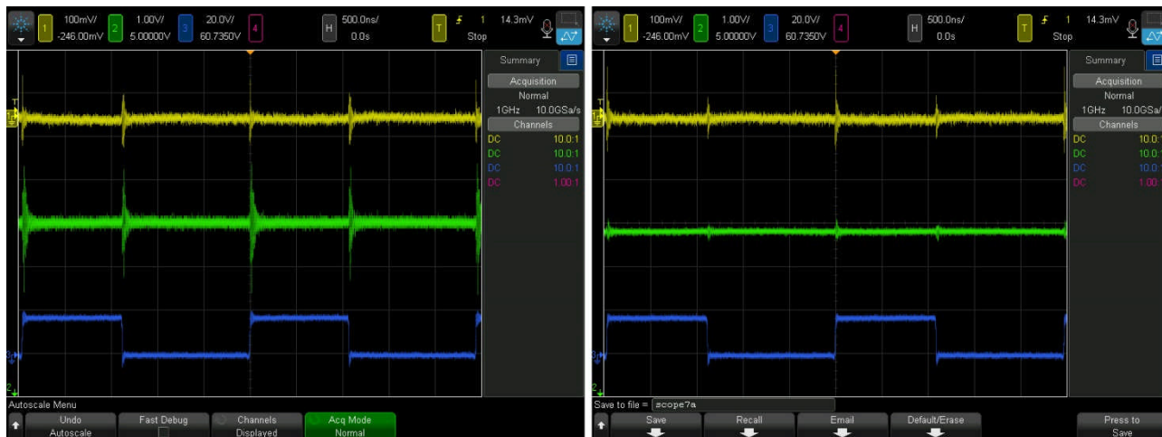
Figure 15: Comparison of unfiltered and filtered Voltages and its filter effect to PARD noise
