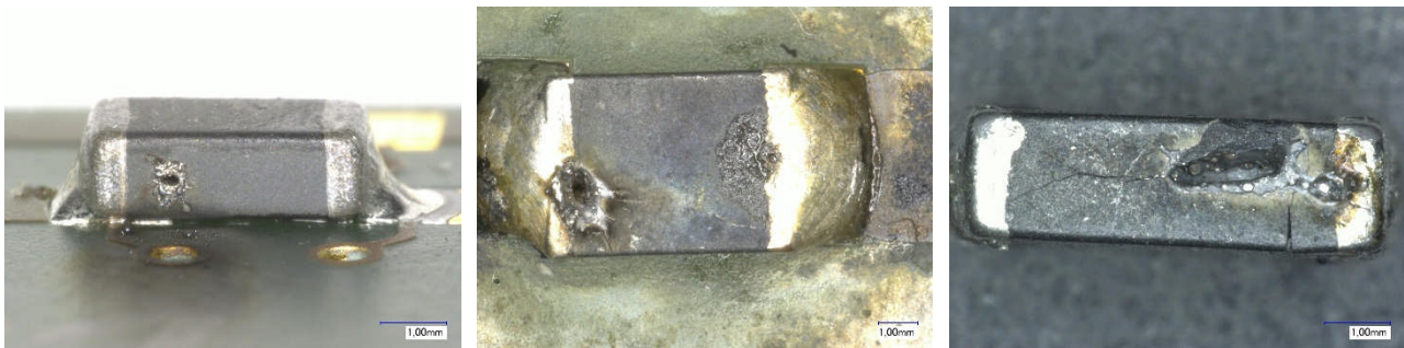
Figure 10: Melted and burned chip bead ferrites due to overcurrent and overheating
