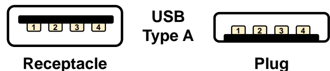
Fig. 1: Pin assignment of the USB interface, type A receptacle and plug
