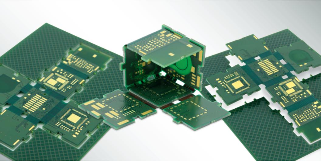
The trend to miniaturization in electronics continues. Integrated circuit board solutions are becoming more and more popular as a means of efficiently utilizing the even smaller casing volume in all three dimensions.
