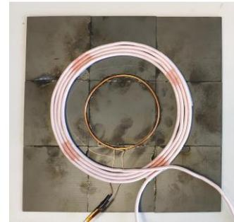
Fig. 7. Prototype of the high power combination coil.
