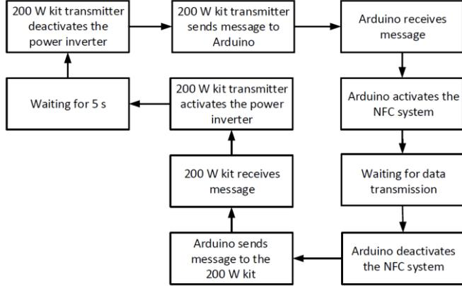
Fig. 6. Workflow of the software to realize a time multiplex procedure.
