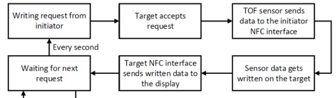
Fig. 4. Workflow of the NFC software.
