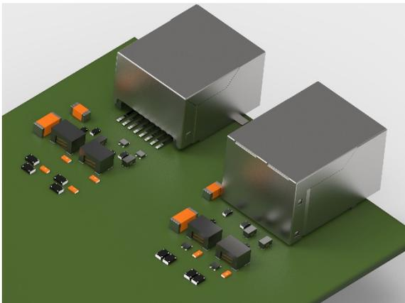
Figure 1: Ethernet PCB with two 100 Base-T connections
