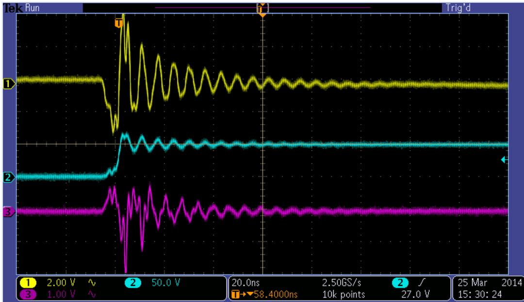
Figure 6: Ringing of the DC501A without any slew rate control.  $V_{IN} = 48V$ ,  $V_O = 12V$ ,  $I_o = 6,0A$
