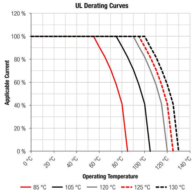
**Figure 3: UL derating curves for different operating temperatures**
