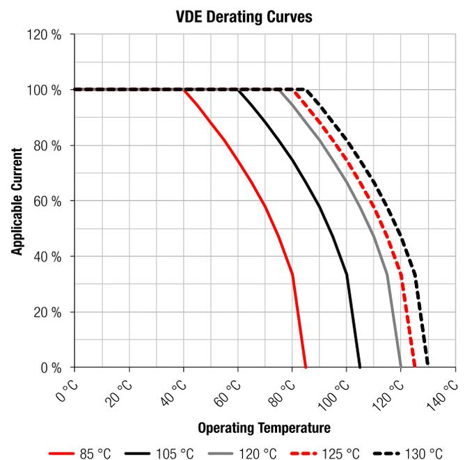
**Figure 4: VDE derating curves for different operating temperatures**
