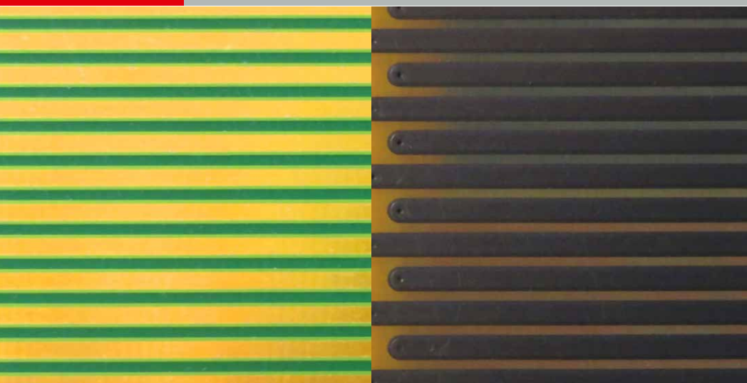
Sensor application with electroplated gold (left) and printed polymer (right)
