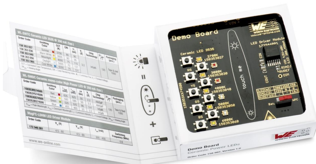
Figure 1: 158 997 Demo Board with part descriptions in packaging
