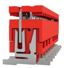
The special fork design of the female socket absorbs relative movements caused by vibration. This prevents fretting corrosion and avoids micro-cuts.
