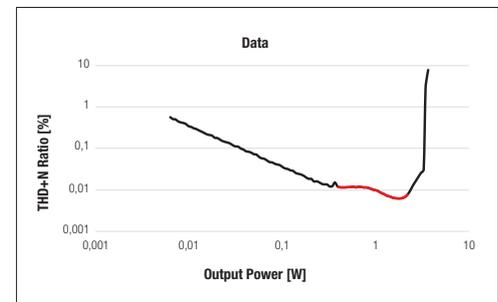
THD+N ratio vs. output power measurement
