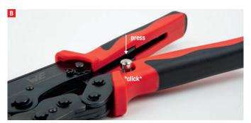
Press the silver button at lower handle, in order to release the crimp head.
