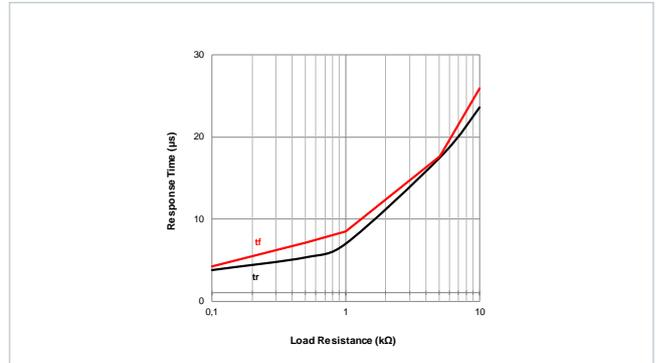
Testcondition:  $I_C = 2mA$ ;  $V_{CE} = 2V$ ;  $T_A = 25^\circ C$
