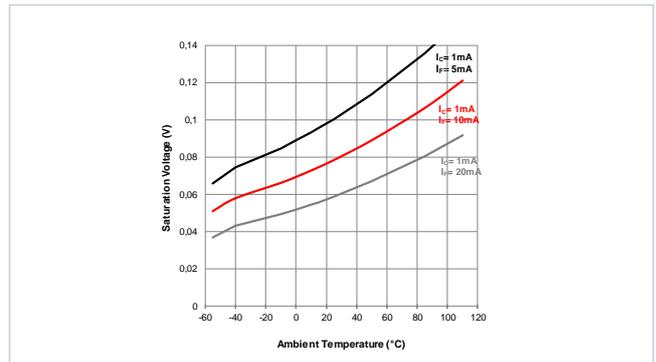
Testcondition:  $I_f = +/- 1mA$ ; Normalized to  $T_A = 25^\circ C$
