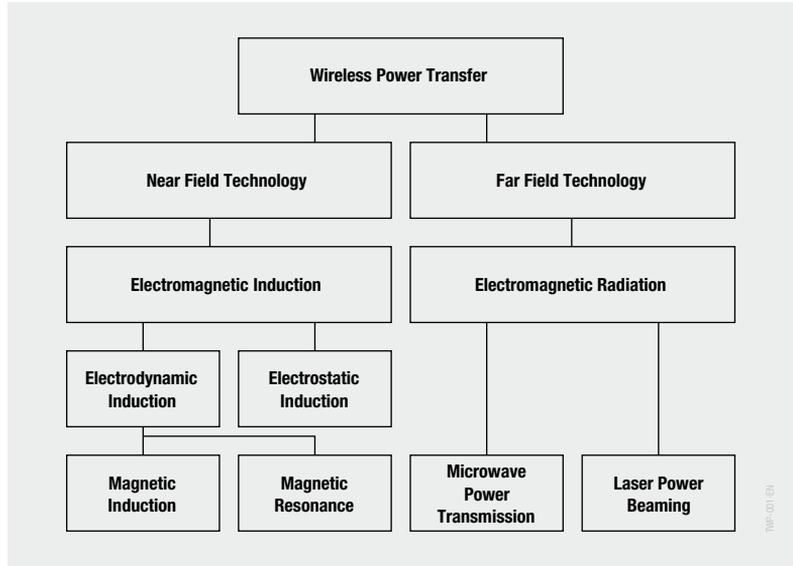
Fig. 1.1: Methods of wireless power transfer
