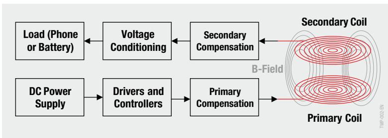
Fig. 1.2: Block diagram of a wireless power transfer system using electromagnetic resonance
