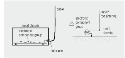
Rod antenna Peripheral cable
