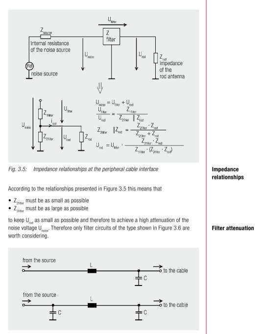
Fig. 3.6: Interface filter circuit versions (common-mode versions not considered)
