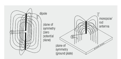
Fig. 3.2: Conversion of the symmetrical dipole to a rod antenna
