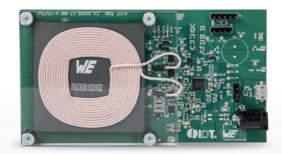
Receiver Module and LED Load Module
