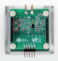
2. Connect your device on those two pads Vout is 12  $\rm V_{DC}$ . Connect your debug connector to J1 for programming
