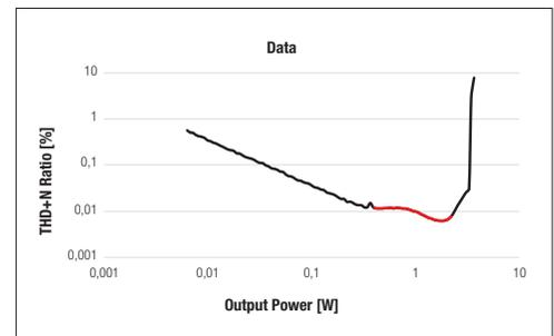
THD+N ratio vs. output power measurement
