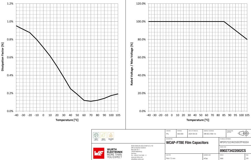
**Rated Voltage vs. Temperature:**
