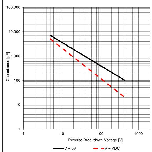
CHECKED REVISION DATE (YYYY-MM-DD) GENERAL TOLERANCE PROJECTION METHOD PeXu 001.003 2023-11-24 DIN ISO 2768-1m HALOGEN **WE-TVSP Power TVS Diode** SMCJ100CA Würth Elektronik eiSos GmbH & Co. KG ORDER CODE EMC & Inductive Solutions WÜRTH Max-Eyth-Str. 1 824541102 74638 Waldenburg **ELEKTRONIK** Germany MORE THAN YOU EXPECT SIZE/TYPE STATUS Tel. +49 (0) 79 42 945 - 0 BUSINESS UNIT PAGE www.we-online.com 3/8 D0-214AB eiSos Valid eiSos@we-online.com
