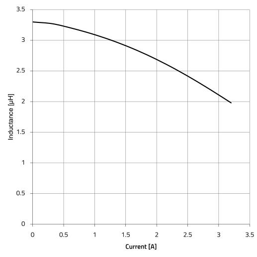
CHECKED REVISION DATE (YYYY-MM-DD) GENERAL TOLERANCE AdGa 003.001 2024-09-16 DIN ISO 2768-1m HALOGEN **WE-MAIA SMT Power Inductor** Würth Elektronik eiSos GmbH & Co. KG ORDER CODE EMC & Inductive Solutions WÜRTH Max-Eyth-Str. 1 78438323033 74638 Waldenburg **ELEKTRONIK** Germany MORE THAN YOU EXPECT SIZE/TYPE STATUS Tel. +49 (0) 79 42 945 - 0 BUSINESS UNIT PAGE www.we-online.com 2/8 2510 eiSos Valid eiSos@we-online.com
