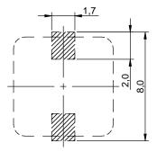
no sensitive traces underneath the component
