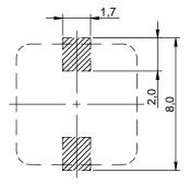
no sensitive traces underneath the component
