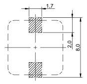
no sensitive traces underneath the component
