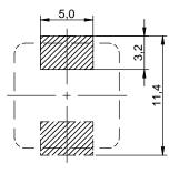
no sensitive traces underneath the component
