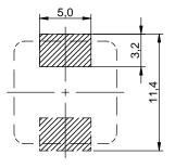
no sensitive traces underneath the component
