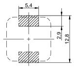
no sensitive traces underneath the component
