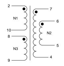
N2 dentotes two windings connected in parallel. Terminals  $4\!+\!5$  and  $6\!+\!7$  must be tied as solder bridging is allowed.
