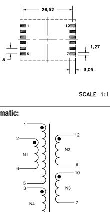
N1 denotes two windings connected in parallel. Terminals 1+2, 5+6 must be tied as solder bridging is allowed.
