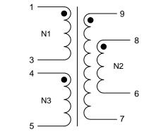
N2 denotes two windings connected in parallel. Terminals 6+7 and 8+9 must be tied as solder bridging is allowed.
