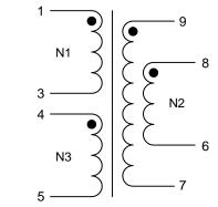
N2 denotes two windings connected in parallel. Terminals 6+7 and 8+9 must be tied as solder bridging is allowed.
