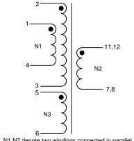
N1,N2 denote two windings connected in parallel. Terminals 1+2, 3+4, 7+8 and 11+12 must be tied as solder bridging is allowed.
