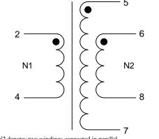
N2 denotes two windings connected in parallel. Terminals 5+6 and 7+8 must be tied as solder bridging is allowed.
