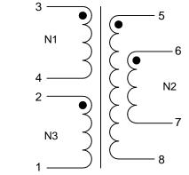
N2 denotes two windings connected in parallel. Terminals 5+6 and 7+8 must be tied as solder bridging is allowed.
