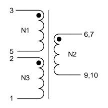
Application of the transformer allows for the leadwires between terminals 6&7 and 9&10 to solder bridge.
