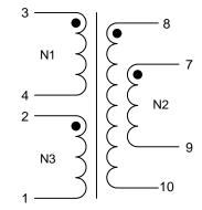
N2 denotes two windings connected in parallel. Terminals 7+8 and 9+10 must be tied as solder bridging is allowed.
