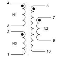
N2 denotes two windings connected in parallel. Terminals 7+8 and 9+10 must be tied as solder bridging is allowed.
