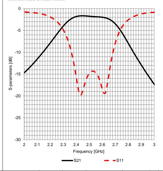
CHECKED GENERAL TOLERANCE PROJECTION METHOD CREATED Würth Elektronik eiSos GmbH & Co. KG **EMC & Inductive Solutions** KaS MuK DIN ISO 2768-1m Max-Eyth-Str. 1 74638 Waldenburg **WE-BPF Multilayer Chip Band-**Tel. +49 (0) 79 42 945 - 0 **Pass Filter** ORDER CODE www.we-online.com 748323024 eiSos@we-online.com DATE (YYYY-MM-DD) BUSINESS UNIT REVISION STATUS PAGE 2018-09-15 3/7 0805 002.000 Valid eiSos **WÜRTH ELEKTRONİK**
