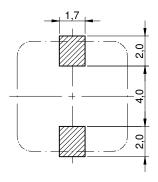
no sensitive traces underneath the component Scale - 2:1
