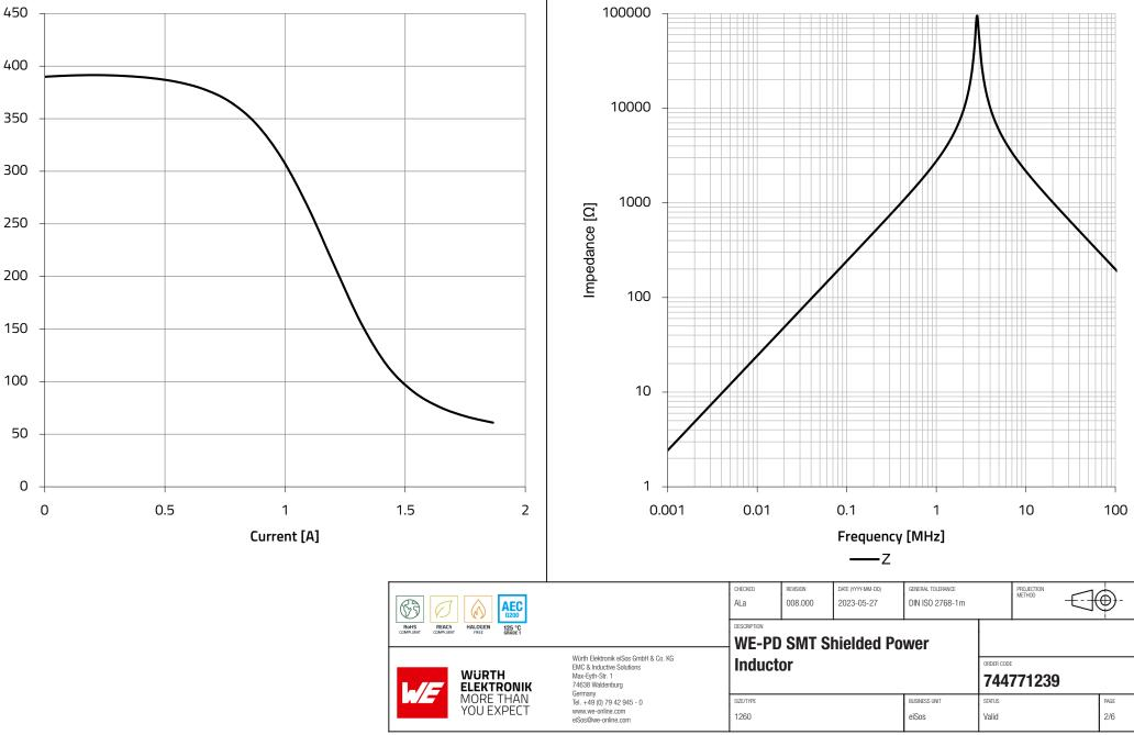
Typical Impedance vs. Frequency Characteristics
