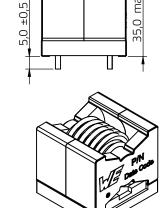
Pin 2 and 3 are only for mechanical stability and are connected to each other.
