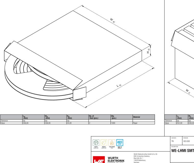
Qty. (pcs.) (mm) Material Inner Carton (pcs.) tvp typ. 354.00 348.00 4000 Paper DATE (YYYY-MM-DD) GENERAL TOLERANCE PROJECTION METHOD  $\oplus$ 2024-12-27 DIN ISO 2768-1m **WE-LHMI SMT Power Inductor** ORDER CODE 7443739650068
