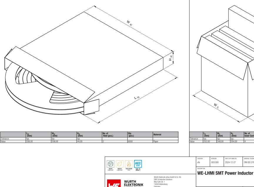
U т νc No. of Qty. (pcs.) w<sub>c</sub> (mm) (mm) Material Inner Carton (pcs.) typ. 354.00 24000 348.00 Paper DATE (YYYY-MM-DD) GENERAL TOLERANCE PROJECTION METHOD
